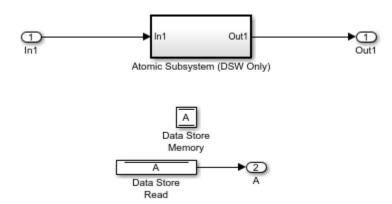
• The subsystem to be extracted contains both Data Store Write and Data Store Read blocks.
