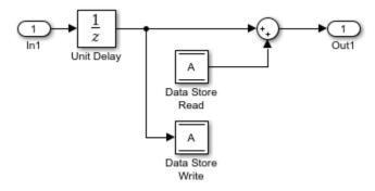
Simulink Design Verifier inserts corresponding Data Store Write blocks with inports into the extracted model.
